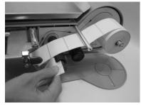
Insert the liner paper into the takeup spindle.
